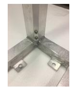
Check 8 bolts to ensure that all are fully tightened.
